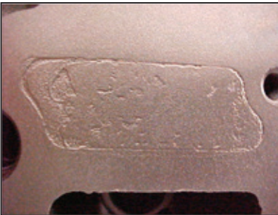
Detail of head face showing pitting in "dead port" area of head gasket.
