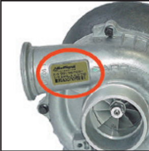
On the compressor housing.
