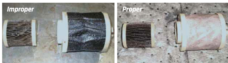
These images show the difference between improperly and properly maintained 6.0L fuel filters
