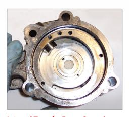
Internal Transfer Pump Corrosion: When the water separator reaches capacity, water flows into the fuel system, causing components such as the internal transfer pump (pictured) to rust. This condition isn't covered under warranty.
