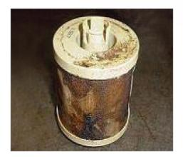
Fuel Filter: A dirty, waterlogged fuel filter (pictured) that does not meet Ford Motor Company specifications can affect the fuel system's ability to separate water from fuel and result in damage that's not covered by warranty.
